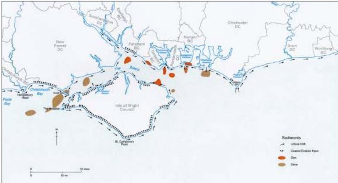
Fig. 7: Sediment transport – inputs, pathways, stores and sinks – of the Isle of Wight.
