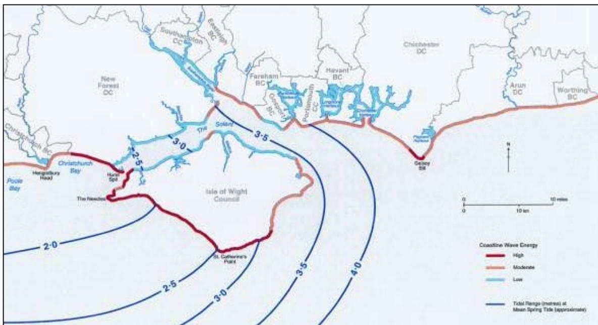
Fig. 6: Tidal currents and wave energy impact on the coast of the Isle of Wight.
