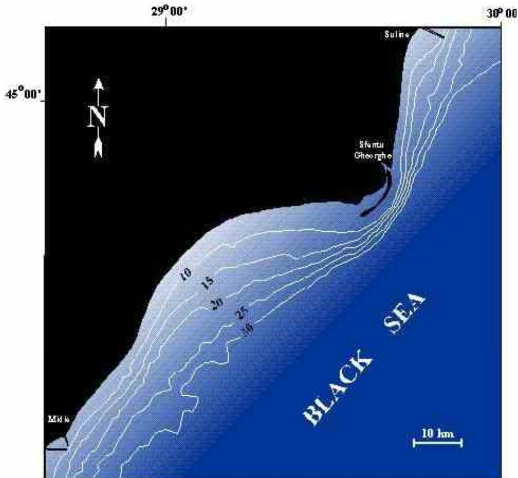
Fig. 4: Nearshore bathymetry of the Danube delta coast.
